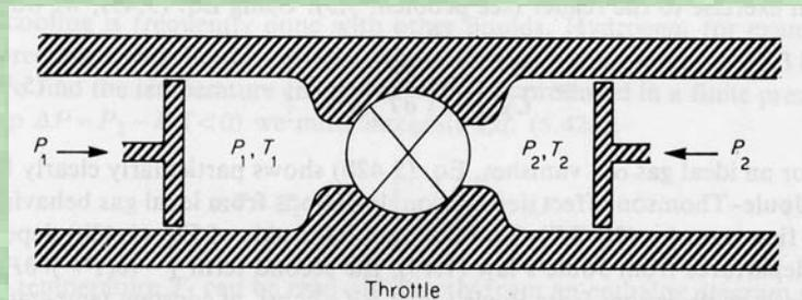
Small mass of gas  $\Delta m$  traverses the obstruction: initial pressure  $p_1$ , volume  $V_1$ , internal energy  $U_1$ ; final pressure  $p_2$ , volume  $V_2$ , internal energy  $U_2$ .
