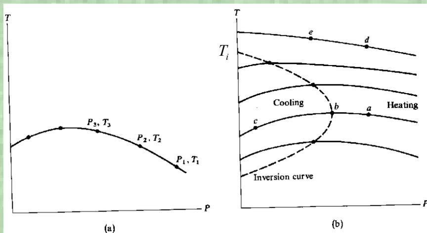
Curves of constant enthalpy. The dashed curve is the inversion curve. On it  $(\partial T/\partial p)_H = 0$ . Inside (outside) it, the gas is cooled (warmed) on expansion.
