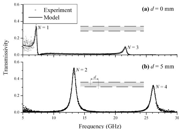
FIG. 3. Experimental frequency-dependent transmissivity data from (a) a structure whose slits on either side of the core are directly opposite each other ( $d = 0$  mm), and (b) a structure with  $d = \lambda_g/2 = 5$  mm. Also shown are the numerically modeled results. Radiation is normally incident ( $\theta = 0^\circ$ ) and detected, and the sample is orientated so that the slit direction is perpendicular to the electric field vector.
